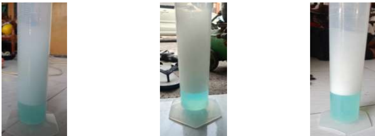
Gambar 3. Hasil Uji :(a) Air50mL Busa210mL (b) Air65mL Busa255mL (c) Air155mL Busa275mL
