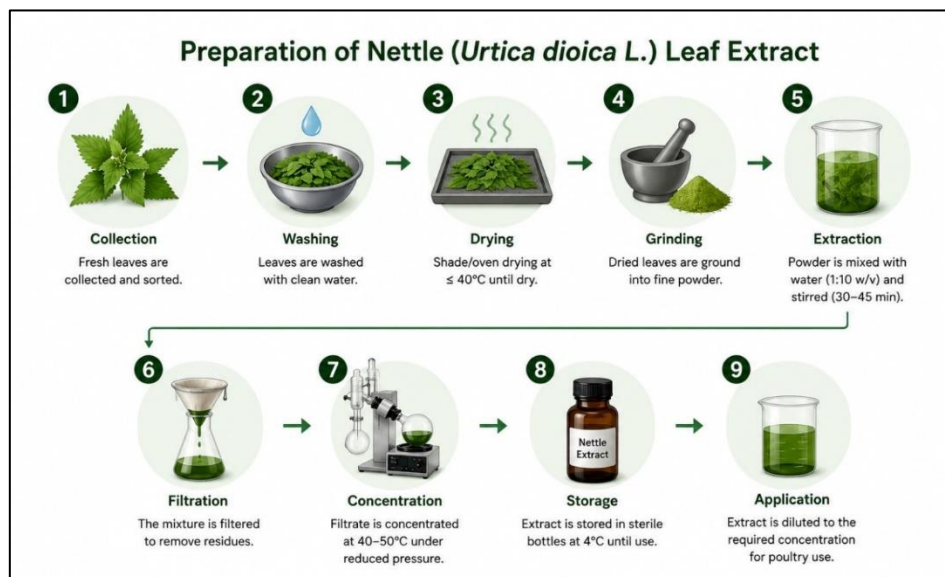
Figure 2. General procedure for aqueous extraction of stinging nettle ( Urtica dioica L.) leaves.
